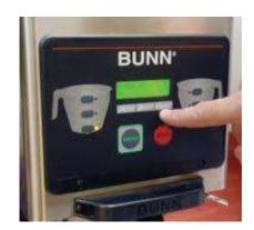
Adjust target grind weight by pressing the (+) or (–)
