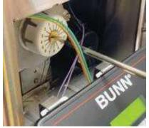
FOR A FINER GRIND: Turn clockwise
